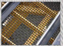
Choose from interchangeable screens from 3/8" (10mm) to 1" (25mm) to quickly remove everything larger than the selected screen hole size.
