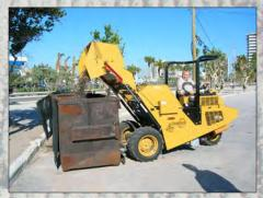
The Model 3000 can ground dump or high lift to 5 ft (152cm) for easy unloading into dumpsters.
